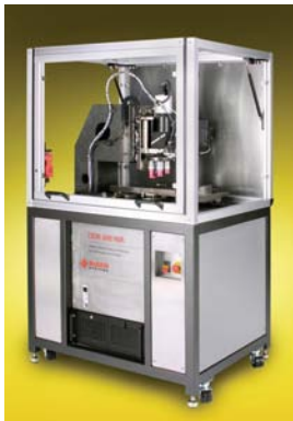
Automated production-floor tools that use NIR technology can detect defects and measure small features inside multilayer MEMS and other chips.
